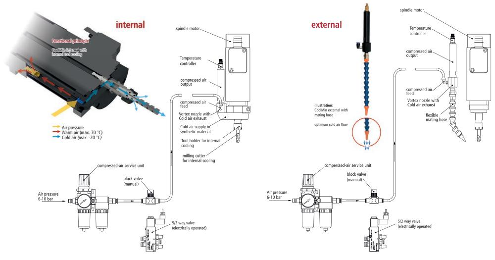
The isel tool cooling system is operated with cold air (up to max. -20°C). In this system, normal operating air (6 up to 10 bar) is used and is freed of dirt particles with a compressedair service unit to prevent icing.
